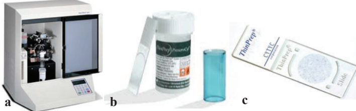
Figure 4 (a): Hologic ThinPrep 2000 machine Figure 4 (b): ThinPrep cytolyt vial for collection of non gynaecological samples, non gynaecological Transcyt blue filter and TP slide Figure 4 (c): PAP stained ThinPrep slide
